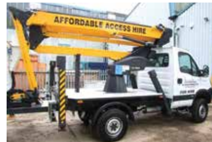
The new 26 metre articulated Co.Me.t Euroskey 26 truck mounted lift
