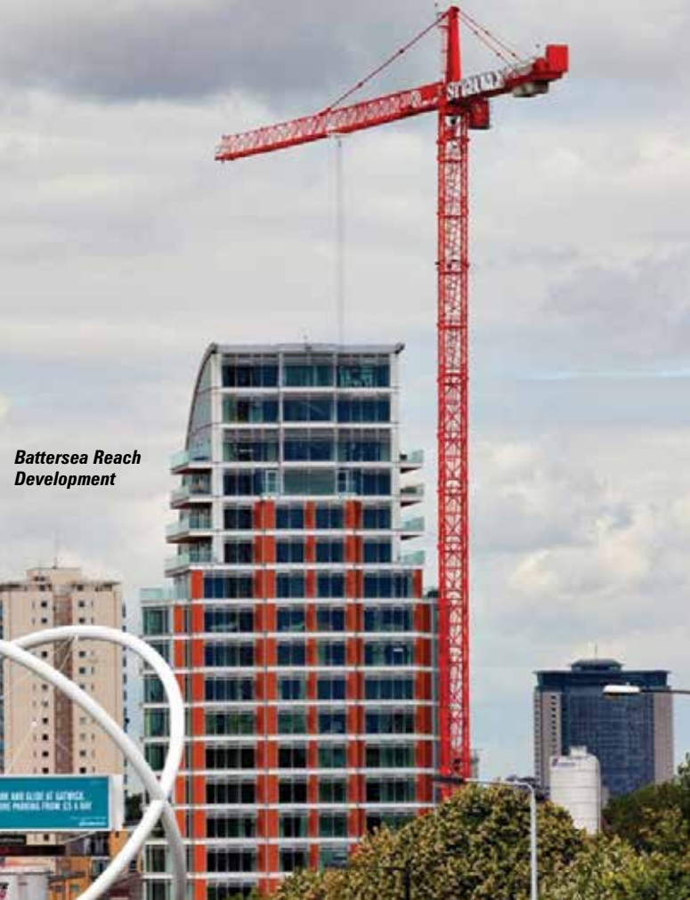
The cranes are also used on demolition contracts - the luffer reduces oversailing problems
