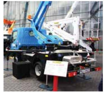
The Palfinger Smart range on a 3.5 tonne chassis now includes this 23.2 metre working height P240A, the P200A, P170T and the P140T.
