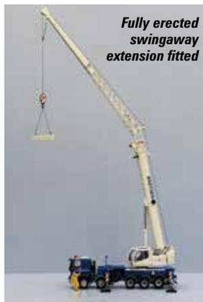
Fully erected swingaway extension fitted
