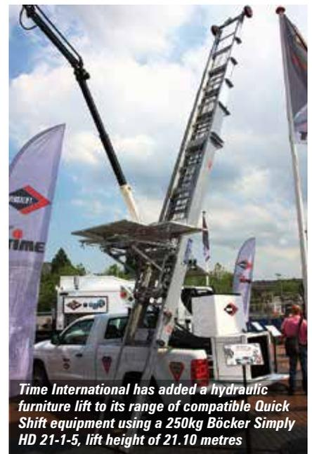
Time International has added a hydraulic furniture lift to its range of compatible Quick Shift equipment using a 250kg Böcker Simply HD 21-1-5, lift height of 21.10 metres
