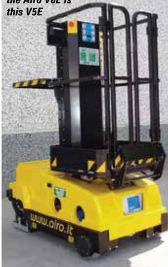
working height of 5.5 metres and a moveable loading platform capable of carrying up to 90kg for stock picking duties.
