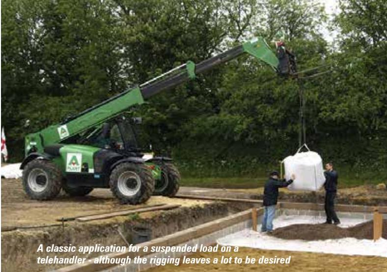
*A classic application for a suspended load on a telehandler - although the rigging leaves a lot to be desired*
