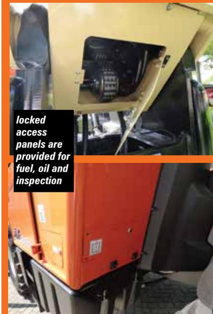
locked access panels are provided for fuel, oil and inspection
