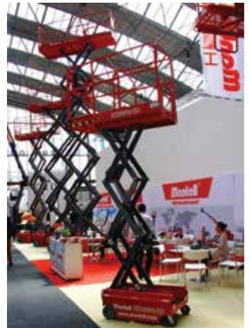
Mantall has several new scissors from seven metres to a 16 metre 1.2 metre wide unit. It is also working on a new range of much lighter straight booms up to 27 metres.
