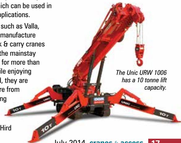
*The Unic URW 1006 has a 10 tonne lift capacity.*
