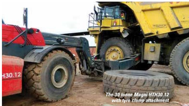
The 30 tonne Magni HTH30.12 with tyre clamp attachment
