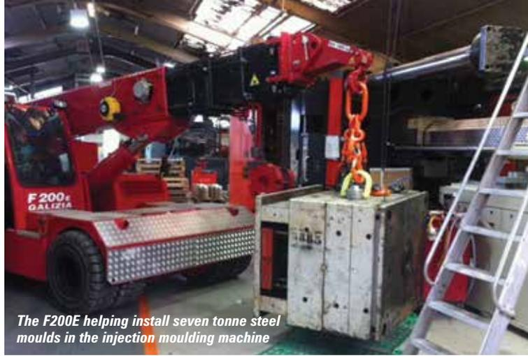
The F200E helping install seven tonne steel moulds in the injection moulding machine
