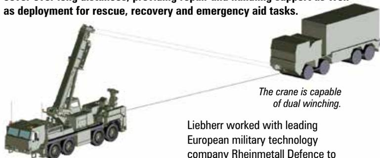
The crane is capable of dual winching.
