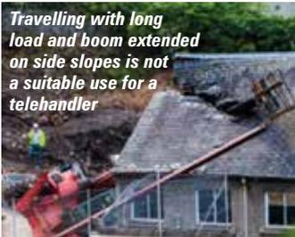
Lifting and travelling with suspended loads is not the primary purpose of a telehandler, so when selecting equipment for this activity the first step should always be to ensure that a telehandler is suitable for carrying out the task safely. Where other equipment is more suitable, it should be used as the
