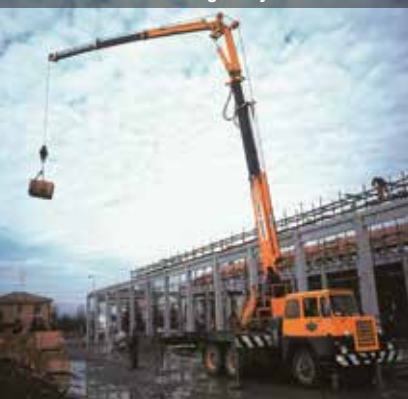
In 1972 the company introduced a 50 tonne/metre crane. With a three section main boom and hydraulically operated three section jib it could reach its 27 metre maximum height in just 28 seconds
