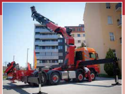
Meister supplied a truck mounted Palfinger PK 200002 L SH loader crane which joined forces with a 53 metre Palfinger WT 530 truck mounted platform
