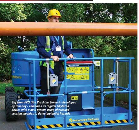
a potential hazard the platform functions stop and the light turns to flashing amber, warning the operator of a potential risk. To re-enable the platform and continue the operator resets the machine's dead-man foot pedal.
