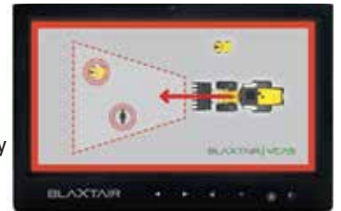
The in cab screen shows pedestrians and other vehicles in addition to emitting an audio alarm
