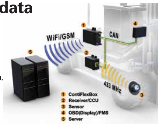
The ContiFlexBox collects the data for onward transmission
