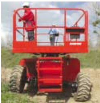
The Manitou 150TP has telehandler type frame levelling.
