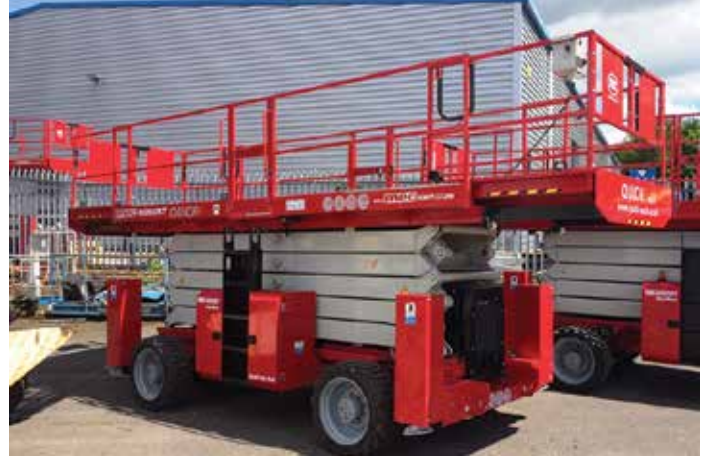
Quick Reach has recently added four 60ft MEC 6092RT Ultra-Decks with 20.5 metre working height and 7.5 metre platform length.
