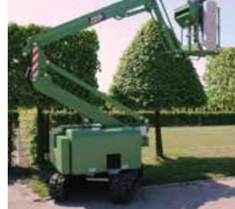
The smallest Custers – a 10 metre tracked boom lift
