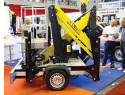
XTRUX which carries out the development work (Co.me.t the sales) has several unusual platforms including this compact trailer unit with just under 12m working height, 4.5m outreach and 200kg.
