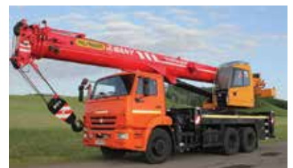
Palfinger Sany's new SPC250 telescopic truck crane mounted on a Kamaz chassis
