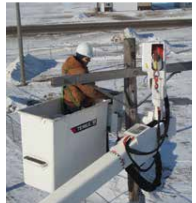
The swing arm combined with the 180 degrees of platform rotation allows an operator to cover both sides of a pole from a single position.
