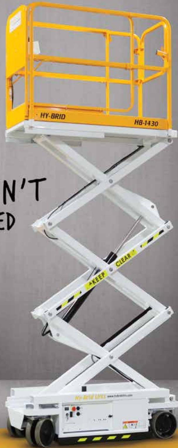
Compact and nimble Hy-Brid Lifts are designed to help you move quickly from one project to the next. With lifting capacities up to 750 pounds and 30-inch slide out deck extensions users have more room, can load more supplies and get more done. The industry leading low floor loading pressures allow them to access green concrete weeks before heavier lifts, and the non-marking wheels won't cause damage to finished floors so they can be on the job from start to finish.
