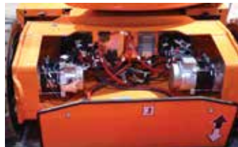
JLG is converting all of its electric booms to direct AC electric drive.
