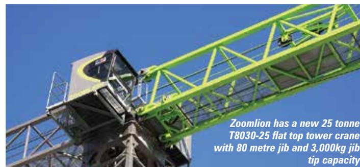
Zoomlion has a new 25 tonne T8030-25 flat top tower crane with 80 metre jib and 3,000kg jib tip capacity
