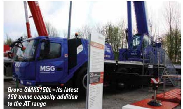
*Grove GMK5150L - its latest 150 tonne capacity addition to the AT range*
