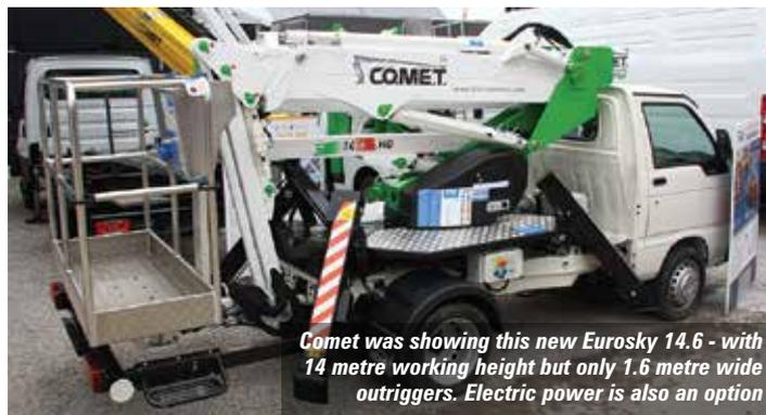
Comet was showing this new Eurosky 14.6 - with 14 metre working height but only 1.6 metre wide outriggers. Electric power is also an option
