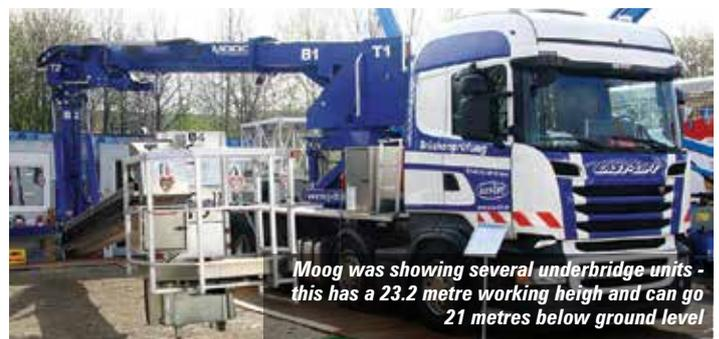
Moog was showing several underbridge units - this has a 23.2 metre working height and can go 21 metres below ground level
