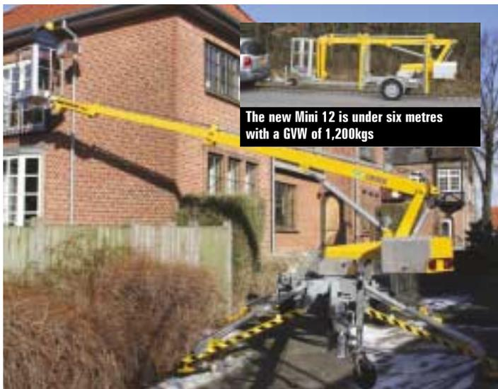
The new Mini 12 is under six metres with a GVW of 1,200kgs
