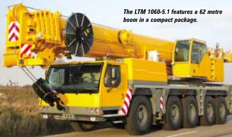
The LTM 1060-5.1 features a 62 metre boom in a compact package.
