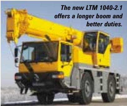
based, and the three axle LTM 1045-3.1. The new crane features a 35-metre, four section full power boom, five metres longer than that of the 1030, (taking it within range of the Terex-PPM AC35L). Its lift capacities are on average around eight percent better than the 1030, rising to 25 percent in the structural part of the chart at higher boom angles.
