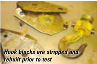
Hook blocks are stripped and rebuilt prior to test
