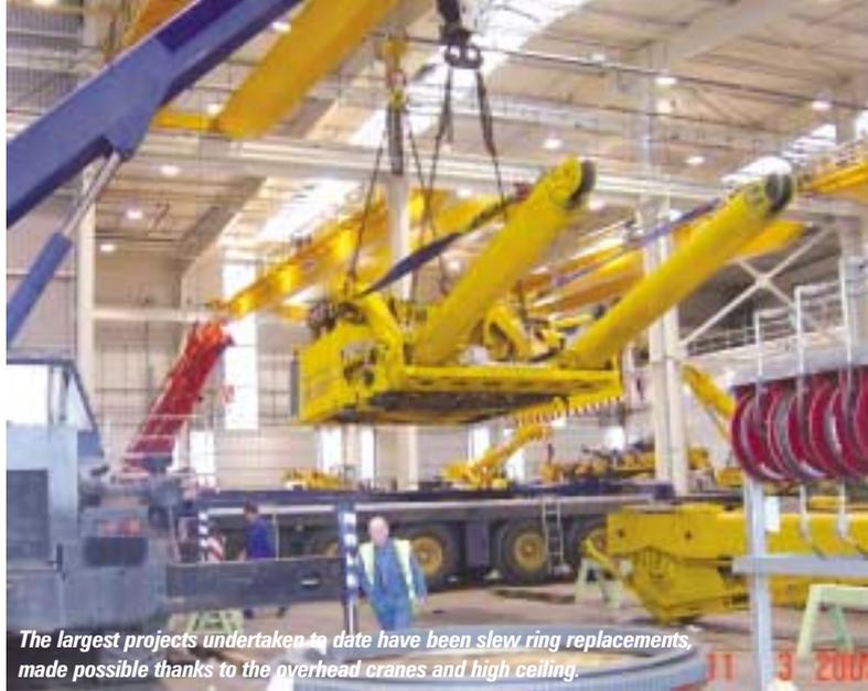
*The largest projects undertaken to date have been slew ring replacements, made possible thanks to the overhead cranes and high ceiling.*
