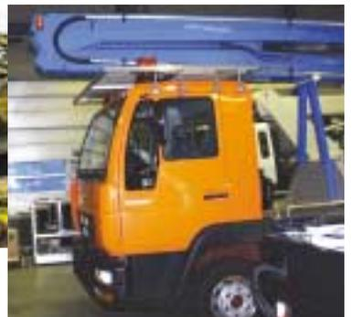
The electrical and hydraulic circuits were almost completely replaced with new as were most of the covers, sheet metal work, platform, gates and railings. Finally this machine was fitted with a new aluminium basket and new control panels. It was then inspected and tested as a new machine with new documentation.
