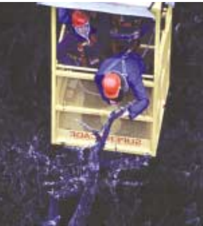
Suspended baskets are used in conjunction with tower cranes for forest canopy research.
