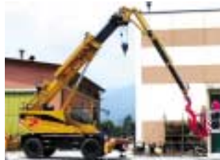
Installations such as this platform fitted to a Locatelli city crane, is governed by EN280 and not the new suspended platform standard
