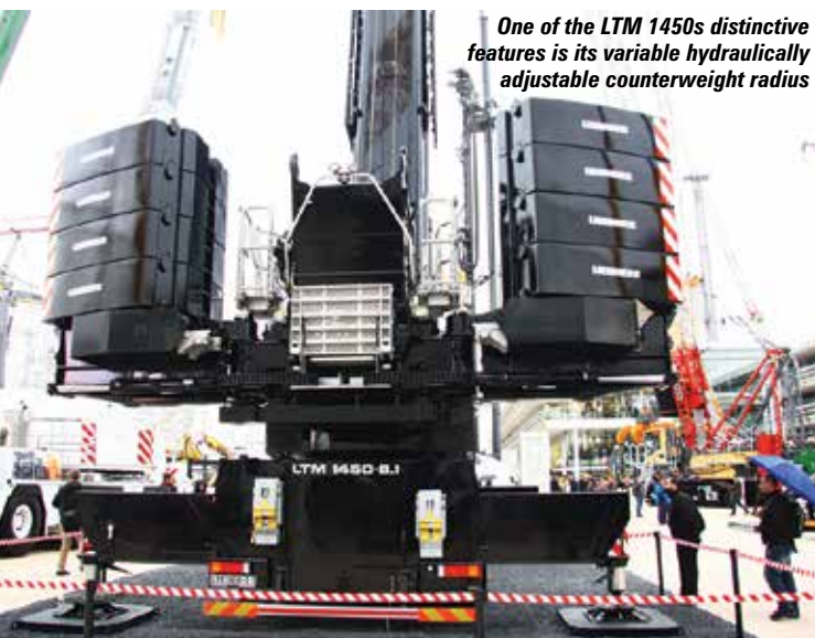
The 450 tonne Liebherr LTM 1450-8.1 designed with 'maximum usability' features an 85 metre boom
