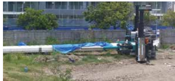
Chris Powell, 41, died when this platform overturned. His 17 year old son was badly injured but survived. Lack of appropriate mats on soft ground caused the overturn.
