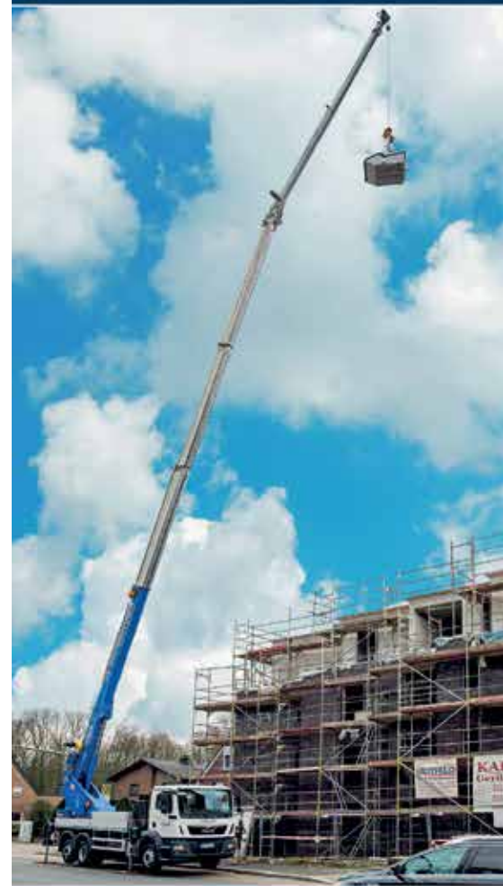
The all-new 13.8m Klubb KAT42 4x4 pick-up mounted lift
