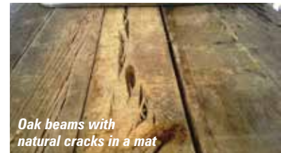
Oak beams with natural cracks and early signs of fungus/mold
