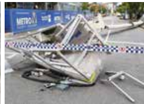
Improper outrigger set-up can be devastating
