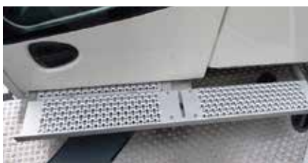
The electrically extendible side platform helps with easy access along with four access ladders to the chassis.
