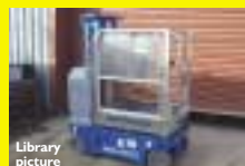
GENIE RUNABOUT GR15 (2005) Self propelled personnel lift. 21' working height. Battery. New old stock. Serviced & tested.
