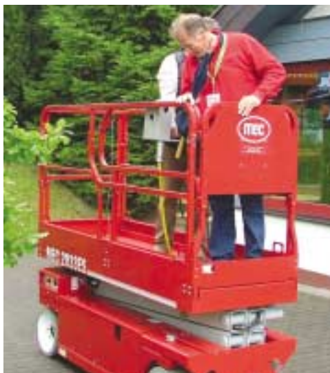
A 20ft scissor offers a long deck and better lift capacities than 19ft models.
