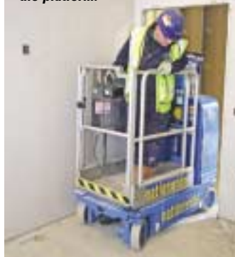
The Runabouts can be driven through regular doorways from the platform.
