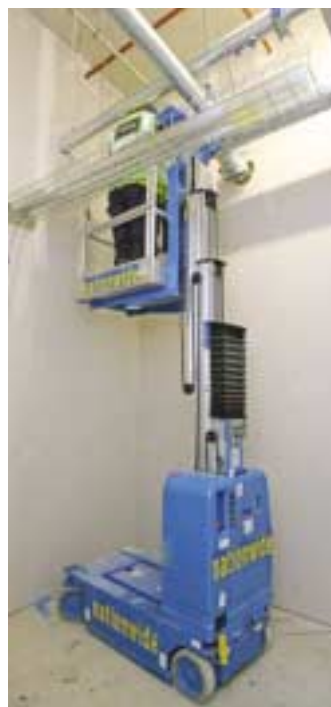
The Genie GR15 is able to access areas too tight for conventional scissors.
