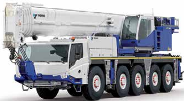
The 110 tonne ATF110-G5 has been upgraded to include multiple counterweight configurations making it easier to configure for road travel.
