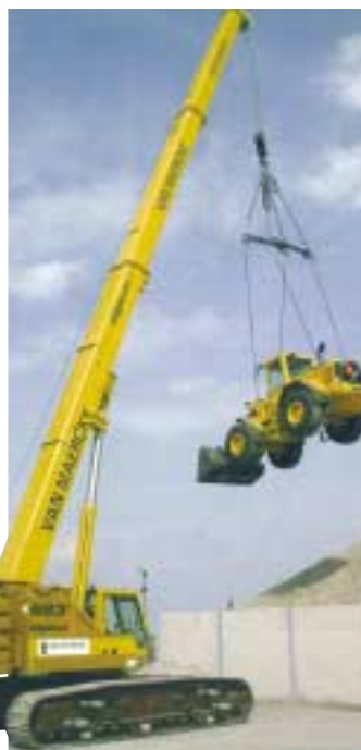
An 80 tonne Heavy duty Sennebogen 683 HD telescopic crawler with 42m boom, owned by Van Marercke of Belgium.
