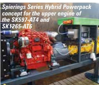
Spierings Series Hybrid Powerpack concept for the upper engine of the SK597-AT4 and SK1265-AT6
