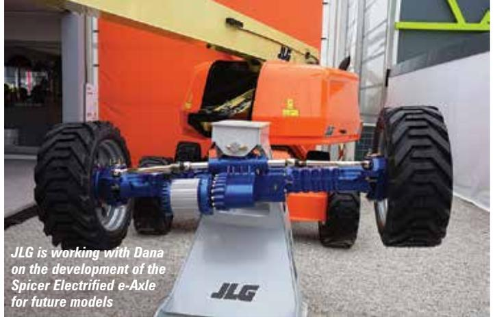
JLG is working with Dana on the development of the Spicer Electrified e-Axle for future models
