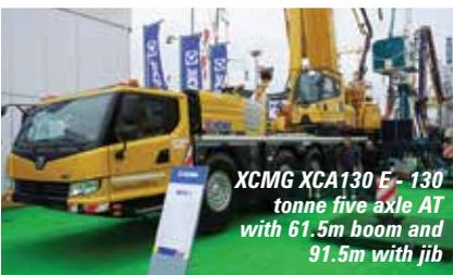
XCMG XCA130 E - 130 tonne five axle AT with 61.5m boom and 91.5m with jib
