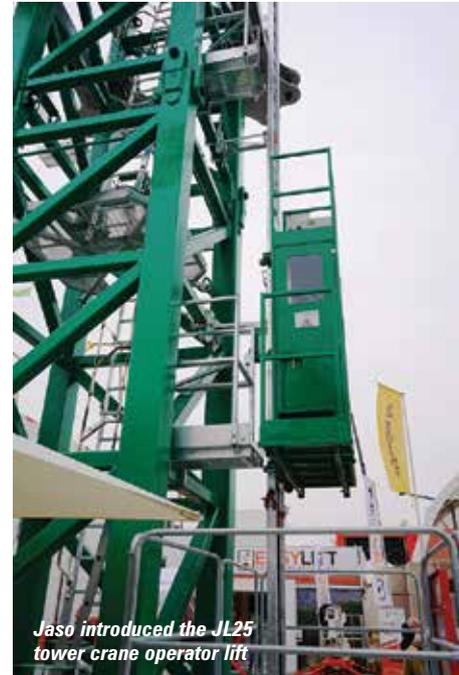
*Jaso introduced the JL25 tower crane operator lift*
