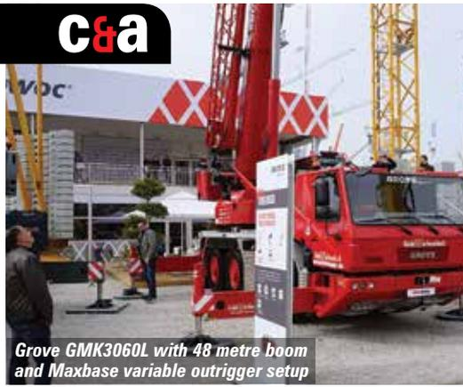
Grove GMK3060L with 48 metre boom and Maxbase variable outrigger setup
