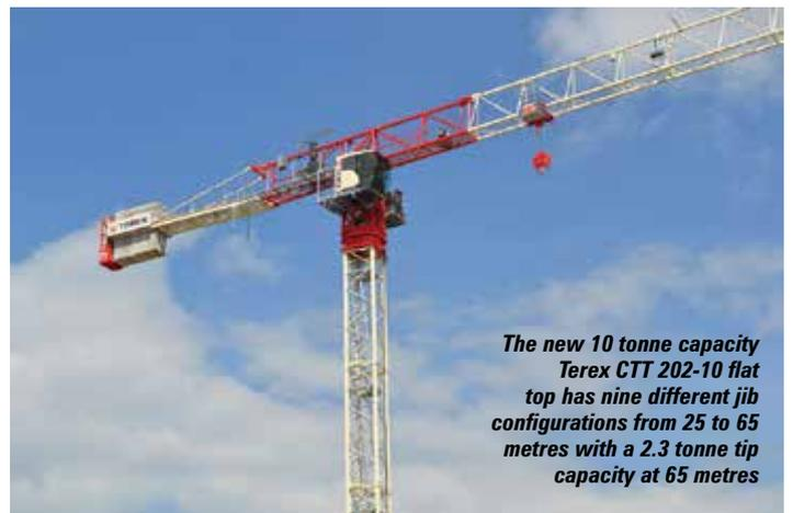
*The new 10 tonne capacity Terex CTT 202-10 flat top has nine different jib configurations from 25 to 65 metres with a 2.3 tonne tip capacity at 65 metres*
