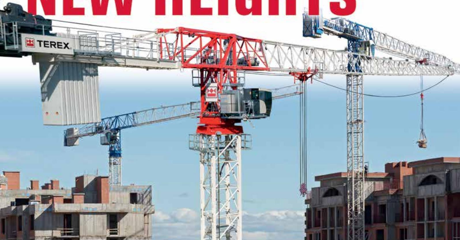
CIT 472-20 Flat Top | Max. lifting capacity of 20 t with 4:1 at the end of the jib.
