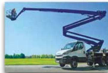
Aerial Platform with a working height of 31 m to be driven with Licence B(E)
