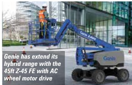
Genie has extend its hybrid range with the 45ft Z-45 FE with AC wheel motor drive
