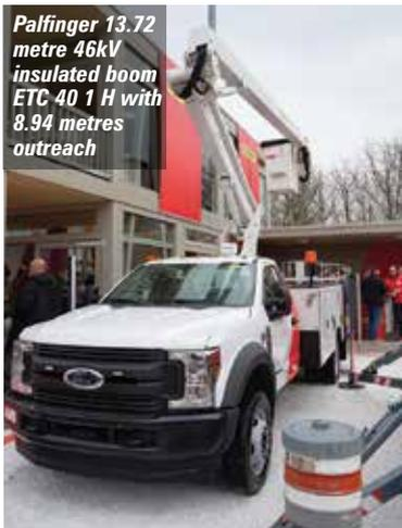
Palfinger 13.72 metre 46kV insulated boom ETC 40 1 H with 8.94 metres outreach
