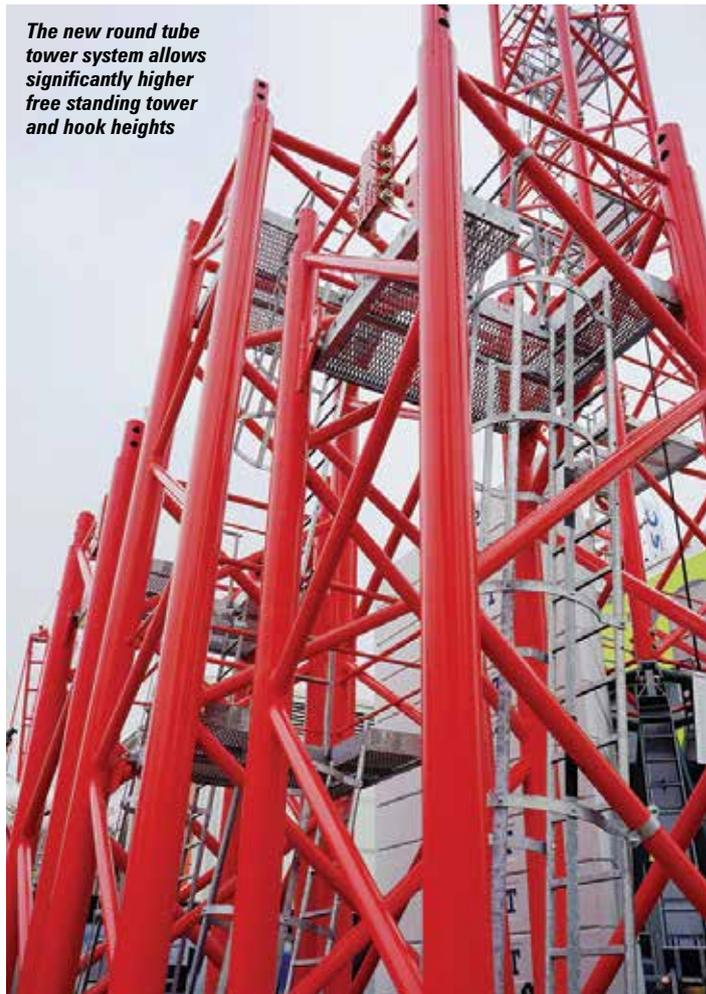
tower elements, while maximum jib lengths of up to 85 metres are available in 2.5 metre increments. The new control and drive
