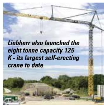
*Liebherr also launched the eight tonne capacity 125 K - its largest self-erecting crane to date*
