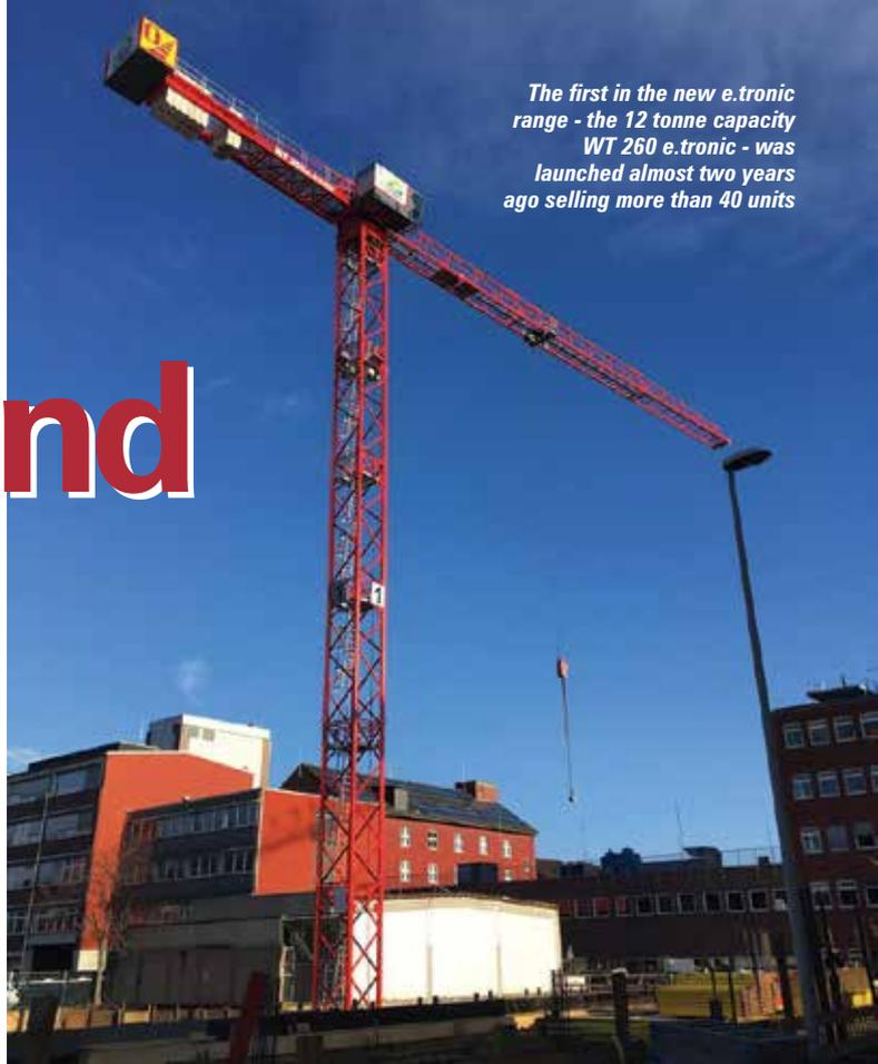
The new round tube tower system allows significantly higher free standing tower and hook heights
