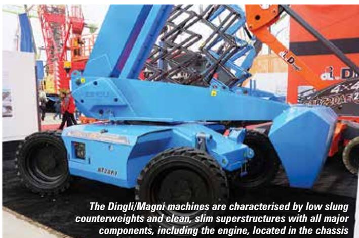
The Dingli/Magni machines are characterised by low slung counterweights and clean, slim superstructures with all major components, including the engine, located in the chassis
