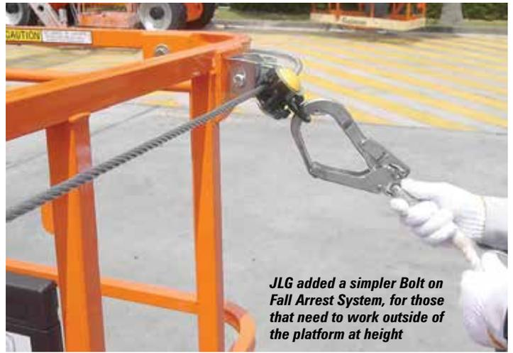
JLG added a simpler Bolt on Fall Arrest System, for those that need to work outside of the platform at height
