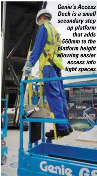
**Genie's Access Deck is a small secondary step up platform that adds 560mm to the platform height allowing easier access into tight spaces**
