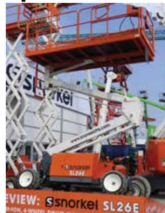
Snorkel has also launched a battery electric version of its 26ft Speed Level SL26 RT with lithium ion battery pack, the Speed Level SL26E. The new machine is said to have sufficient battery power for a full day's work and offers the same gradeability and speeds as the diesel model. A remote 2.5kWh single phase battery charger can recharge the battery pack to 80 percent within 20 minutes, while the onboard charger takes 6.5 hours to full charge.
