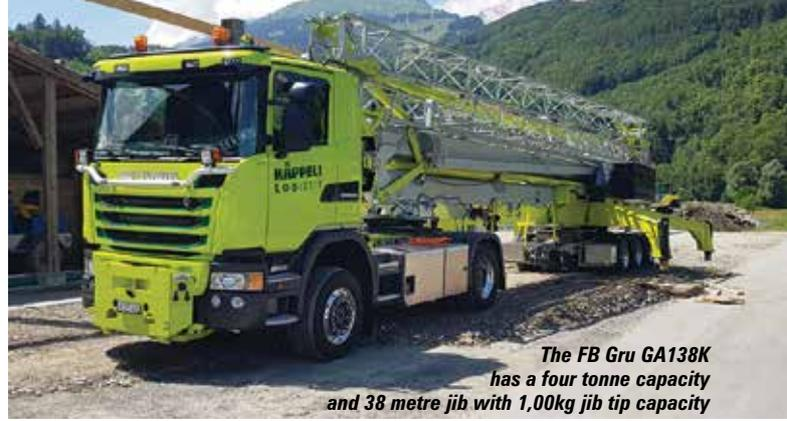
*The FB Gru GA138K has a four tonne capacity and 38 metre jib with 1,00kg jib tip capacity*
