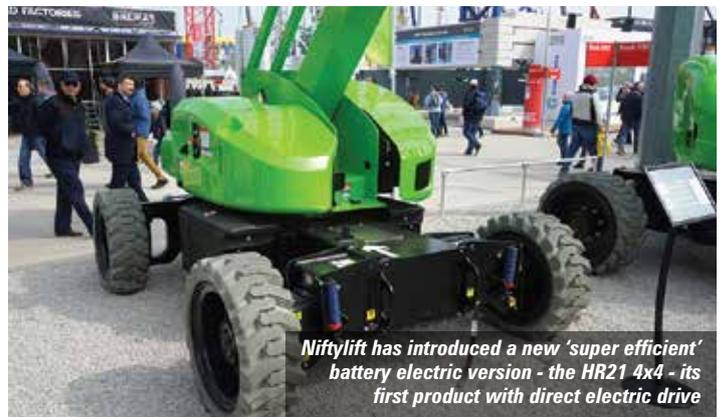
Niftylift has introduced a new 'super efficient' battery electric version - the HR21 4x4 - its first product with direct electric drive
