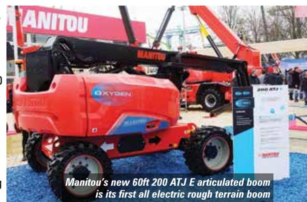
Manitou's new 60ft 200 ATJ E articulated boom is its first all electric rough terrain boom
