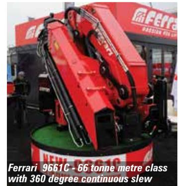
Ferrari 9661C - 66 tonne metre class with 360 degree continuous slew
