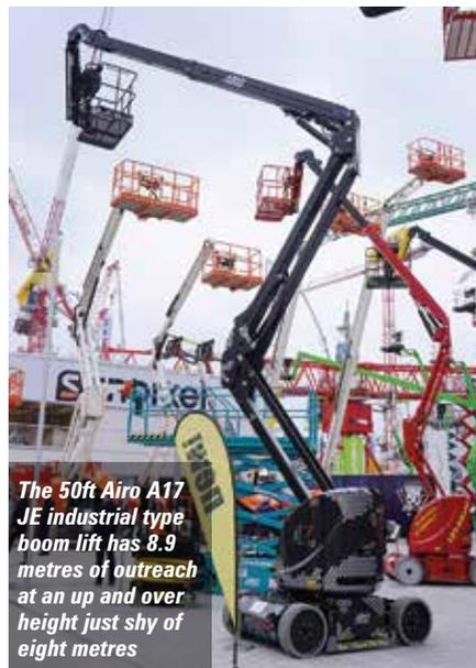
The 50ft Airo A17 JE industrial type boom lift has 8.9 metres of outreach at an up and over height just shy of eight metres
