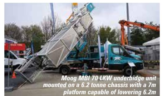
Moog MBI 70 LKW underbridge unit mounted on a 6.2 tonne chassis with a 7m platform capable of lowering 6.2m
