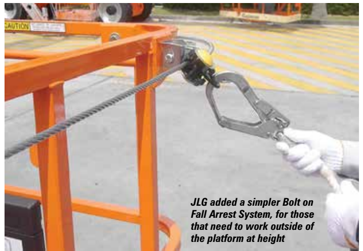
The system consists of two steel brackets connected by a 1.8 metre steel cable with a sliding ring to which a harness lanyard can be clipped
