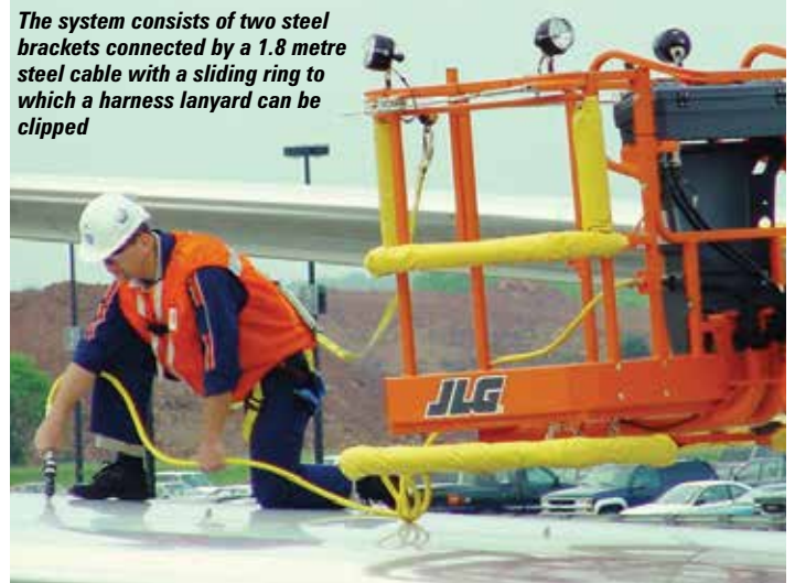
JLG added a simpler Bolt on Fall Arrest System, for those that need to work outside of the platform at height
