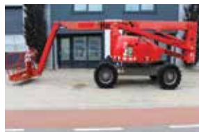
HAULOTTE - HA20PX Articulating boom lifts Diesel, 4x4x4 Drive, 20.0m Working Height, 2008 | PHM-Id 09085
