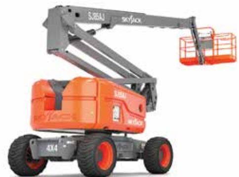
Largest of Skyjack's articulated booms the SJ85 AJ has a 27.9 metre working height and just over 17 metres of outreach.
