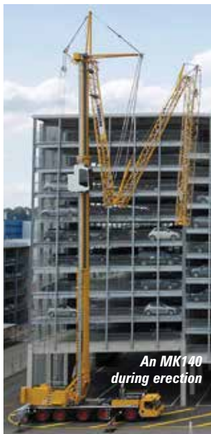
The Liebherr MK140 can luff up to 70 degrees giving a hook height of 94.4 metres
