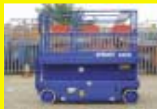
UPRIGHT X26N (1992) Self propelled scissor lift. 32' working height. Battery. Repainted, serviced & tested.
