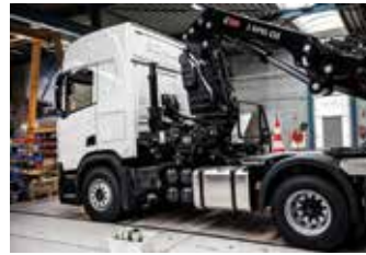
Hiab BodyWorks - for heavy cranes - significantly reduces installation time.
