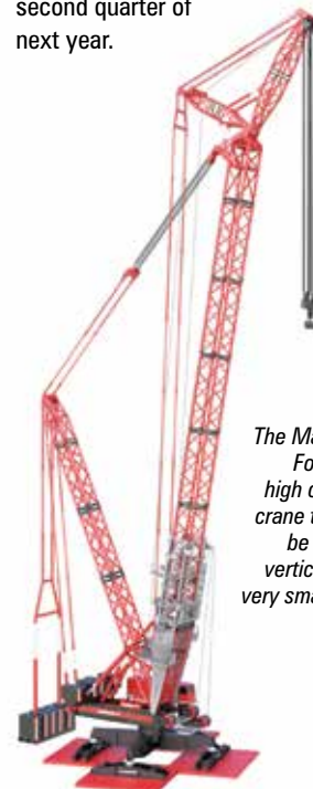
ALE adapted a Manitowoc 18000 crawler crane to significantly reduce the contract time for the installation of 16 wind turbines
