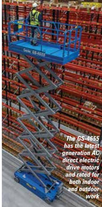
The GS-4655 has the latest generation AC direct electric drive motors and rated for both indoor and outdoor work
