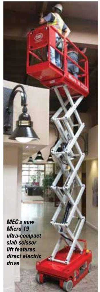
MEC's new Micro 19 ultra-compact slab scissor lift features direct electric drive
