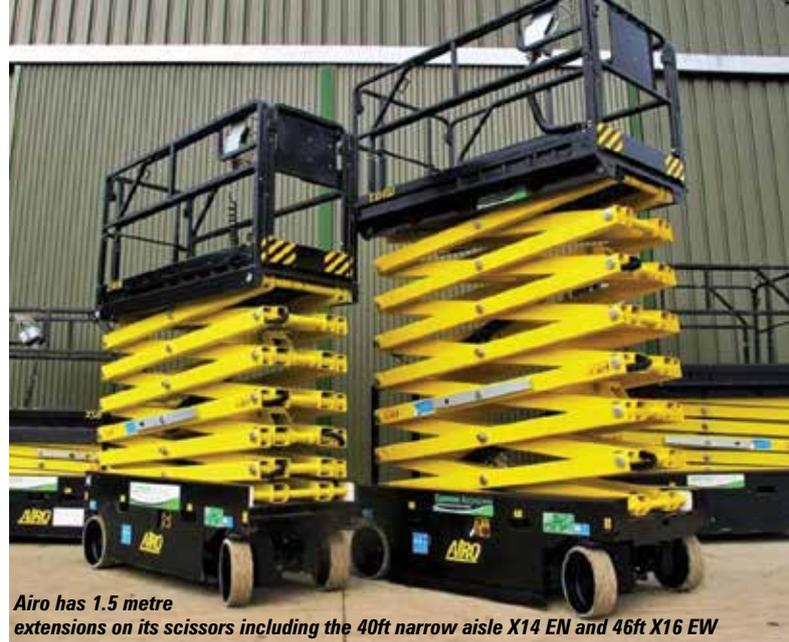
Airo has 1.5 metre extensions on its scissors including the 40ft narrow aisle X14 EN and 46ft X16 EW
