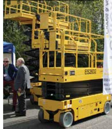
capacity of 750kg and can drive at heights of up to 20 metres. However it will not tolerate slopes of more than one degree so built-in inboard levelling jacks will automatically level the machine on ground that is off level or uneven. The new platform has clearly been designed for installation, maintenance and cleaning work within high cube warehousing, although it might struggle to move down the narrow aisles.
