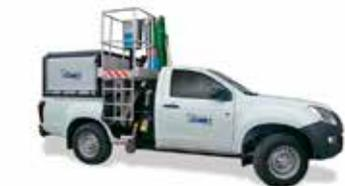
Platforms to work in height combined to the functionality of the Pick-up.
