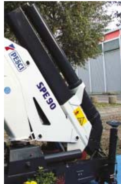
This Pesci crane is unusual in that it uses a minimal open base section.
