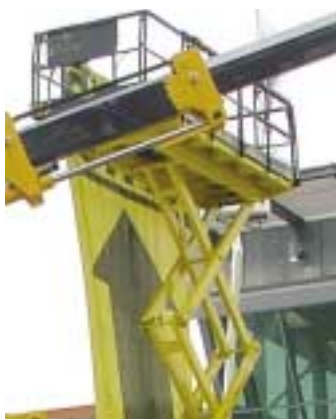
It is light but large objects that cause the most danger to a scissor lifts stability, such as this huge banner.
