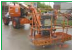
SELF PROPELLED TELESCOPIC PLATFORM 2000 JLG 450AJ 15m. working height (51ft.). Deutz Diesel. Choice of several machines.
