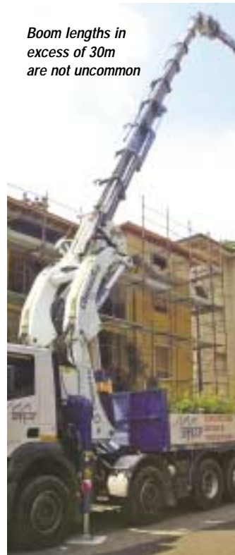
This Pesci crane is unusual in that it uses a minimal open base section.
