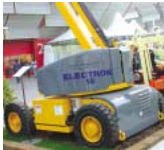
Basket's 16 metre Electron battery powered boom
