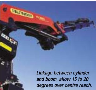
Linkage between cylinder and boom, allow 15 to 20 degrees over centre reach.
