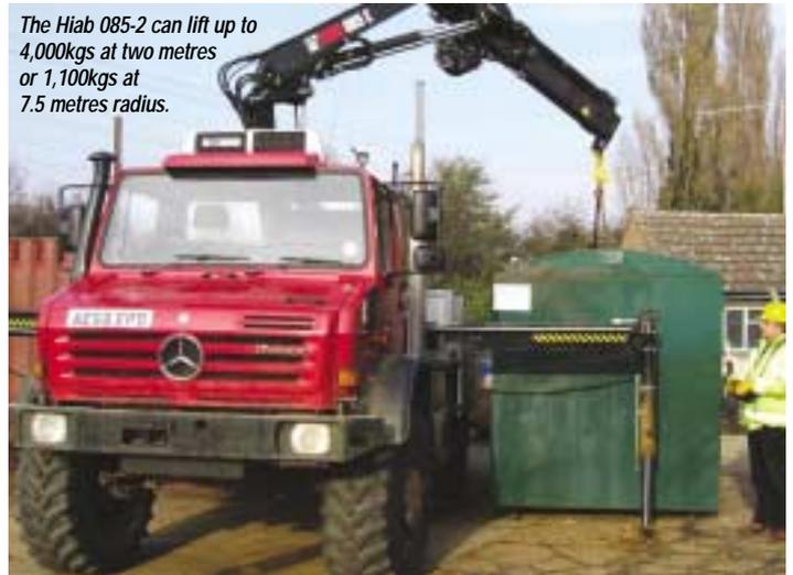
The Unimog 5000 is matched to a Hiab 085-2 crane, giving 1,110 kgs lift capacity at 7.5 metres and a tip height of around nine metres. The cranes compact, profile takes up less than 700mm of space, ideal for the Unimog's short (3.85m) wheelbase, leaving a reasonable amount of space for cargo. Its low height of 2.1 metres, is also important, given that this vehicle already stands tall, thanks to its over generous ground clearance.
