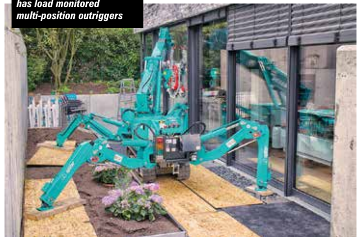
The PCC 115.002 is Palfingers largest articulated crawler crane
