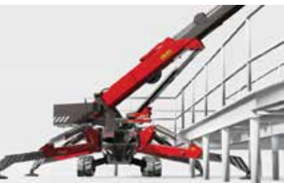
The Hoeflon C30e has a five section main boom topped by an optional five section telescopic luffing jib.
