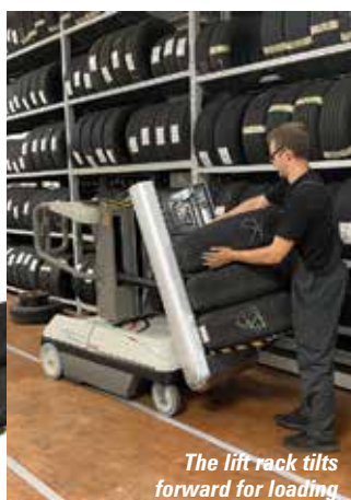
The lift rack moves to horizontal so that tyres can be rolled off or onto shelving
