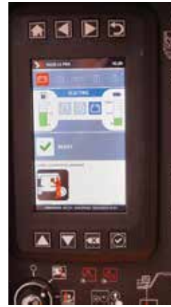
Part of the HA20 LE's control panel showing fuel and battery charge remaining.
