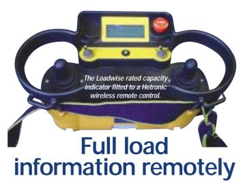
Loadwise, working with Hetronic, has introduced a new system for wireless remote controls for cranes. The system provides a full suite of information to the operator, within a small LED window on the Hetronic shoulder strap controller. This fully satisfies the latest standards that demand that rated capacity indicator data is continuously available to the operator, including a warning of approaching overload, given in terms of percentage of rated capacity and allowable radius with given load.
