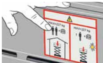
One of the main differences is the effect of wind loading when applied to stability tests and calculations. Here is an example of an A92.20 decal.
