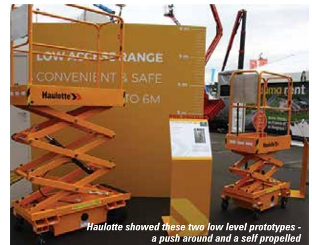
Haulotte showed these two low level prototypes - a push around and a self propelled
