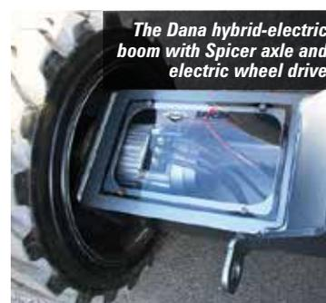
The Dana hybrid-electric boom with Spicer axle and electric wheel drive
