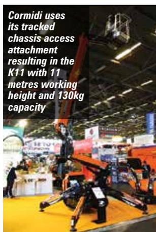
Cormidi uses its tracked chassis access attachment resulting in the K11 with 11 metres working height and 130kg capacity
