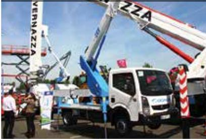
ELS launched its new 10.2m VM10-J mast boom with 3.15m outreach, 200kg capacity, 990mm width and weighing 2,600kg
