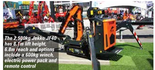
The 2,500kg Jekko JF40 has 8.1m lift height, 6.8m reach and options include a 600kg winch, electric power pack and remote control
