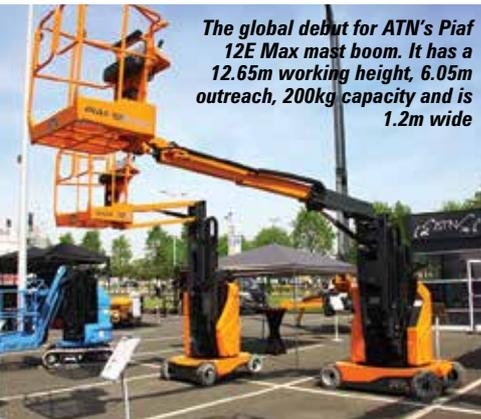
The global debut for ATN's Pif 12E Max mast boom. It has a 12.65m working height, 6.05m outreach, 200kg capacity and is 1.2m wide
