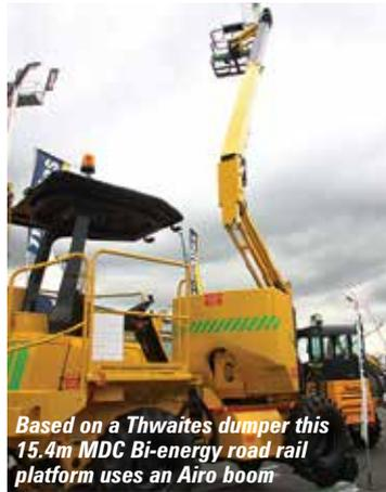
Based on a Thwaites dumper this 15.4m MDC Bi-energy road rail platform uses an Airo boom
