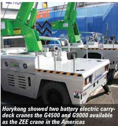
Horykong showed two battery electric carry-deck cranes the G4500 and G9000 available as the ZEE crane in the Americas
