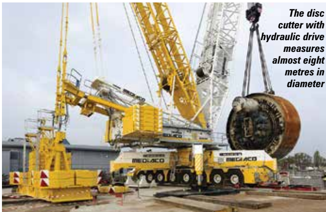
The 150 tonne derrick ballast with a variable radius (shown suspended) was only required for the first phase of the lift
