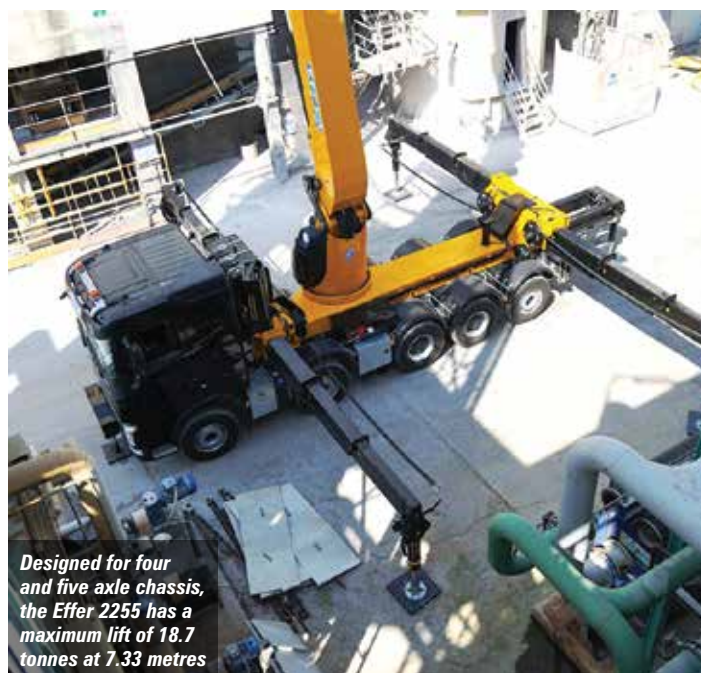
Effer's new flagship model the 2255 has a maximum reach of 55 metres
