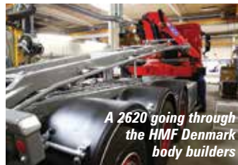
One of the first twin hydraulic control muck away cranes being built at Aarhus
