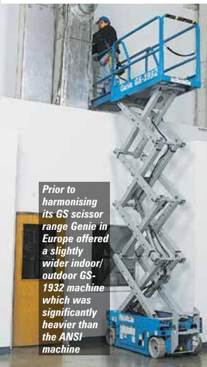
Prior to harmonising its GS scissor range Genie in Europe offered a slightly wider indoor/outdoor GS-1932 machine which was significantly heavier than the ANSI machine
