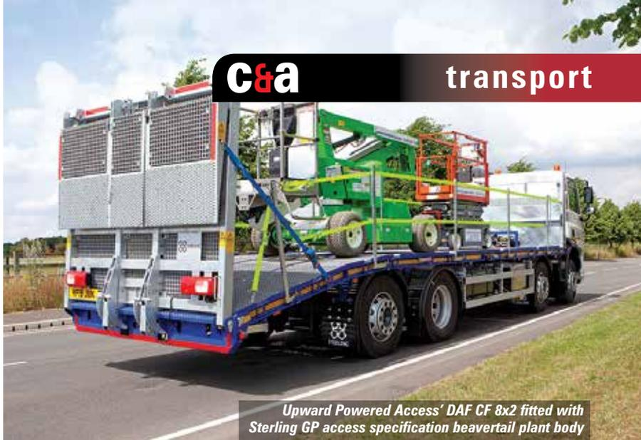
Upward Powered Access' DAF CF 8x2 fitted with Sterling GP access specification beavertail plant body
