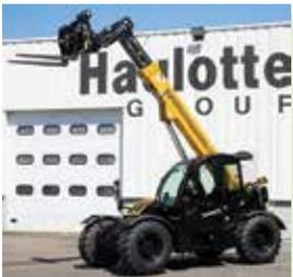
**Haulotte** starts shipping its new 3.2 tonne/seven metre **HTL 3207** telehandler, its most compact unit to date.
