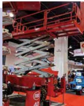
**MEC** unveils two compact battery/diesel Rough Terrain scissiors - the 33ft 3369 RT and 40ft 4069RT - and two straight telescopic boom lifts with articulated jibs - the 45ft 45-J and 65ft 65-J.
