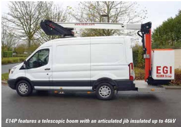
E14P features a telescopic boom with an articulated jib insulated up to 46kV
