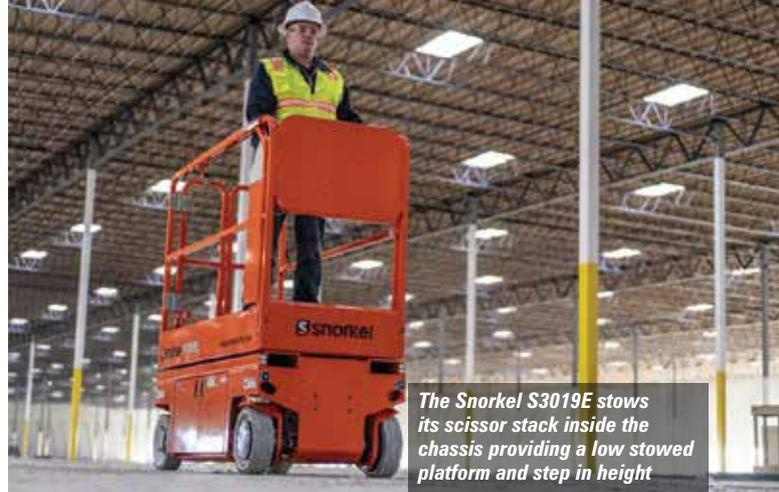
The Snorkel S3019E stows its scissor stack inside the chassis providing a low stowed platform and step in height
