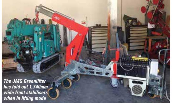
The JMG Greenlifter has fold out 1,740mm wide front stabilisers when in lifting mode
