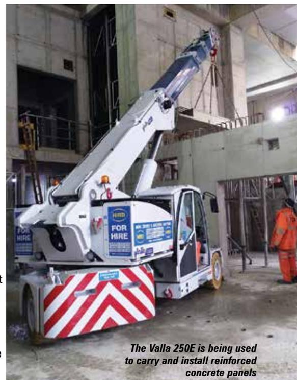
The Valla 250E is being used to carry and install reinforced concrete panels
