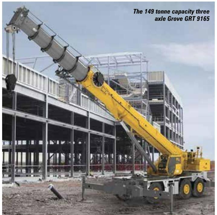
The 149 tonne capacity three axle Grove GRT 9165
