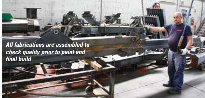
All fabrications are assembled to check quality prior to paint and final build
