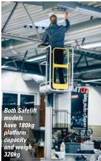
Both Safelift models have 180kg platform capacity and weigh 320kg
