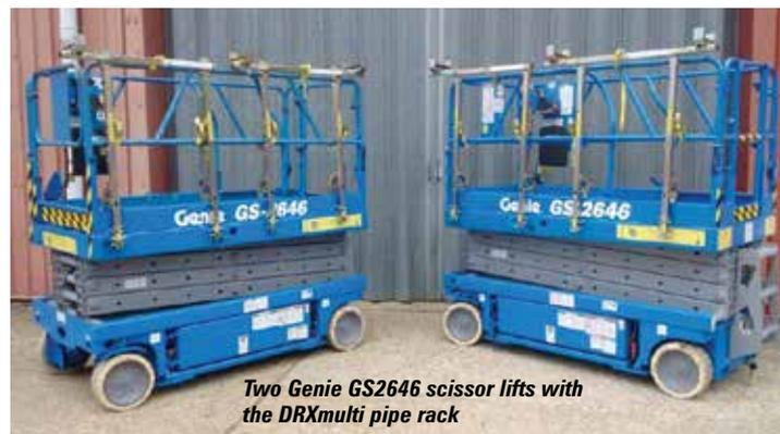
Two Genie GS2646 scissor lifts with the DRXmulti pipe rack
