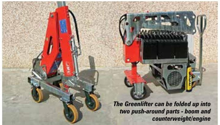
The Greenlifter can be folded up into two push-around parts - boom and counterweight/engine
