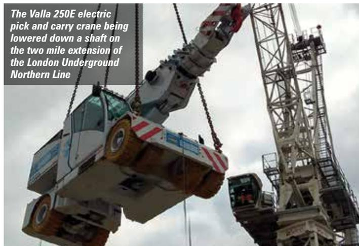
The Valla 250E electric pick and carry crane being lowered down a shaft on the two mile extension of the London Underground Northern Line
