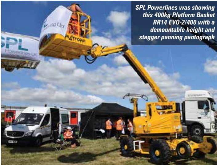
SPL Powerlines was showing this 400kg Platform Basket RR14 EVO-2/400 with a demountable height and stagger panning pantograph
