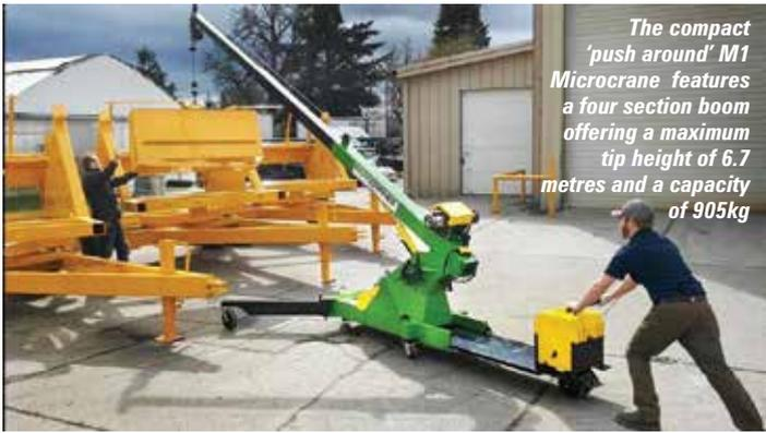
The compact 'push around' M1 Microcrane features a four section boom offering a maximum tip height of 6.7 metres and a capacity of 905kg
