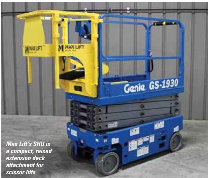
Man Lift's SHU is a compact, raised extension deck attachment for scissor lifts
