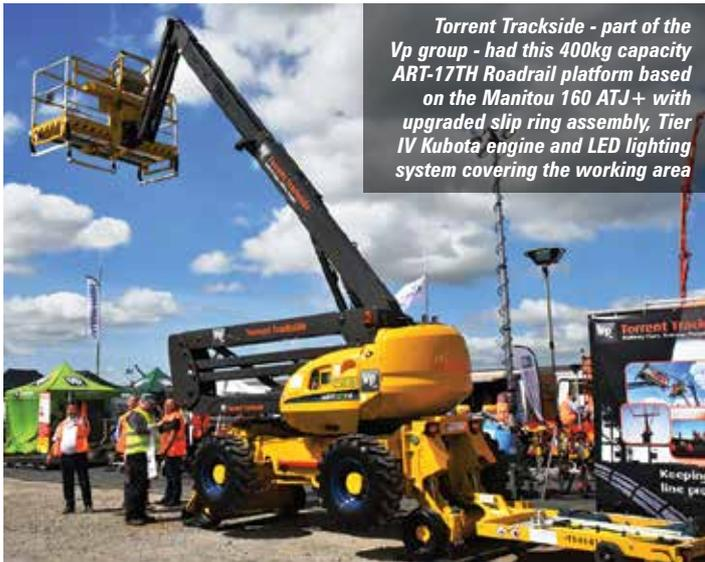
Torrent Trakside - part of the Vp group - had this 400kg capacity ART-17TH Roadrail platform based on the Manitou 160 ATJ+ with upgraded slip ring assembly, Tier IV Kubota engine and LED lighting system covering the working area
