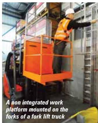
A non integrated work platform mounted on the forks of a fork lift truck
