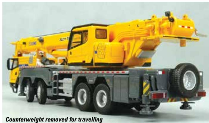
*Counterweight removed for travelling*
