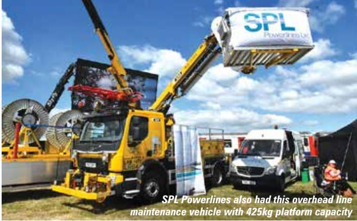
SPL Powerlines also had this overhead line maintenance vehicle with 425kg platform capacity
