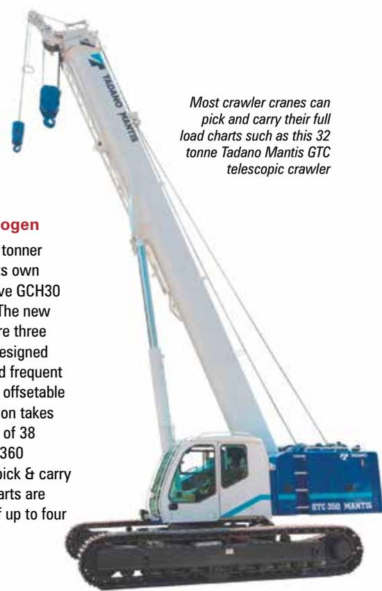
Most crawler cranes can pick and carry their full load charts such as this 32 tonne Tadano Mantis GTC telescopic crawler
