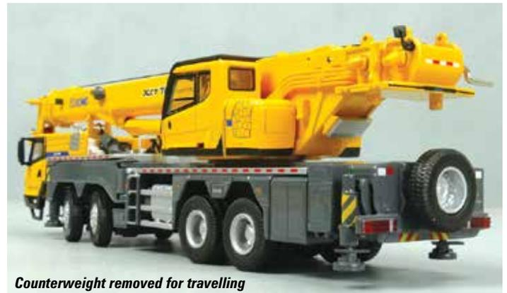
*Counterweight removed for travelling*
