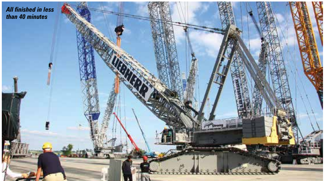
6. Next the boom is lifted into position
