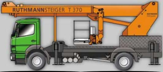
+++37 m working height+++28 m outreach+++8,8 m total length+++500 kg cage load+++
