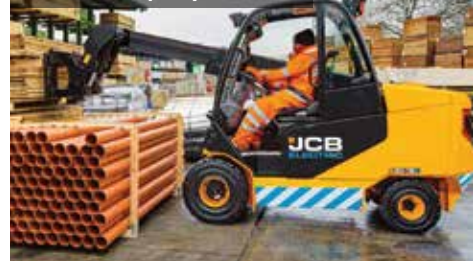
JCB's new C30-19e Teletruck has a four metre lift height with up to three tonnes capacity
