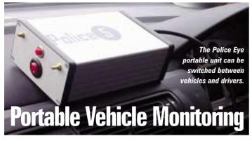
Logistic companies are already using vehicle and driver tracking and monitoring systems to improve their efficiency and cut costs. To date only a few Crane or Access rental companies have employed this technology, Police5 Technologies has now launched an Eye-TraX portable unit. The Eye-TraX Portable provides high accuracy location and reliable 'on-demand' GPRS communications via the Web in a light weight, compact, transferable unit that does not need hard wiring into a vehicle.
