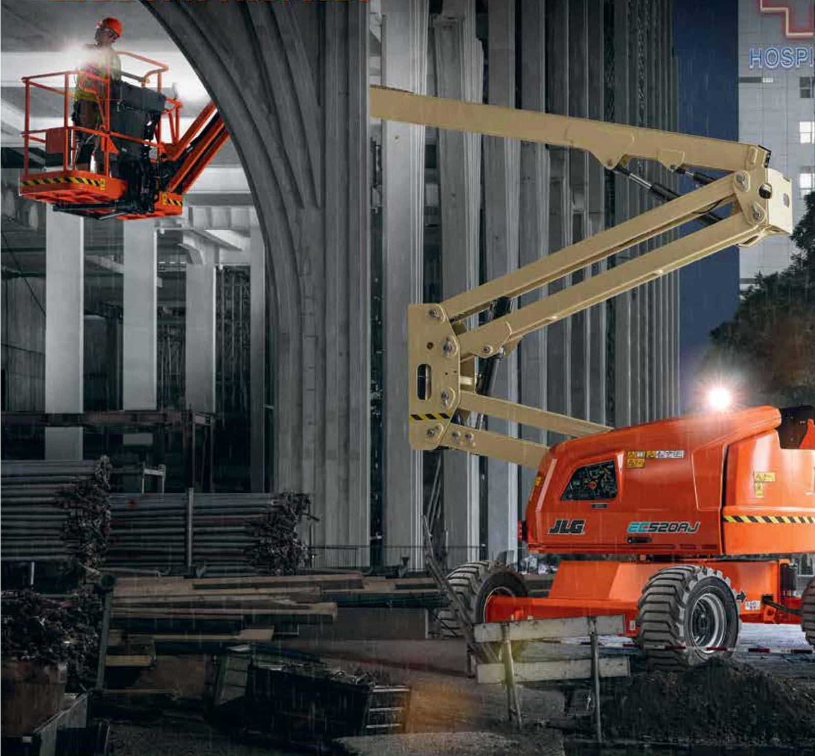
Now you can work in sensitive areas without disrupting the surrounding environment. Powered by safe, quick-charging lithium ion batteries and two electric motors, JLG® EC booms deliver clean operation and greater energy efficiency on any job site. Experience uncompromised performance with the flexibility to work inside or out with a single machine.
