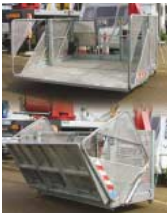
The roofers platform option on the Oil&Steel 35m Eagle truck mount.
