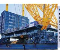
Sarens launches the largest landbased crane in the world - the 5,000 tonne, 250,000 tonne/ metre SGC-250 capable of lifting 2,000 tonnes at 100 metres.
