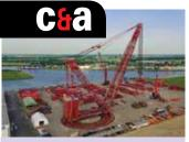
Mammoet upgrades its 3,200 tonne, 200,000 tonne/metre PTC 200DS modular ring crane to the 210,000 tonne/metre PTC 210 DS.
