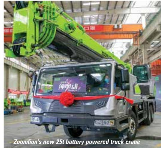
Zoomlion's new 25t battery powered truck crane
