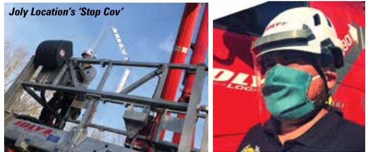
maintain separation and shield against microscopic projections, covering the full height and width of the platform. The polycarbonate material is said to be "ultra-transparent, flexible, scratch resistant and unbreakable". It also has operators with face shields for their helmets, masks and gloves, while platforms are equipped with hand sanitiser stations.
