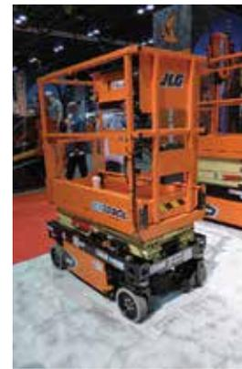
the market with a line of Chinese built scissor lifts. It has introduced a number of innovations, especially at this end of the market. Its 1930ED has a good all-round specification and an excellent folding guardrail set up which truly is easy to operate and rugged enough to remain that way.
