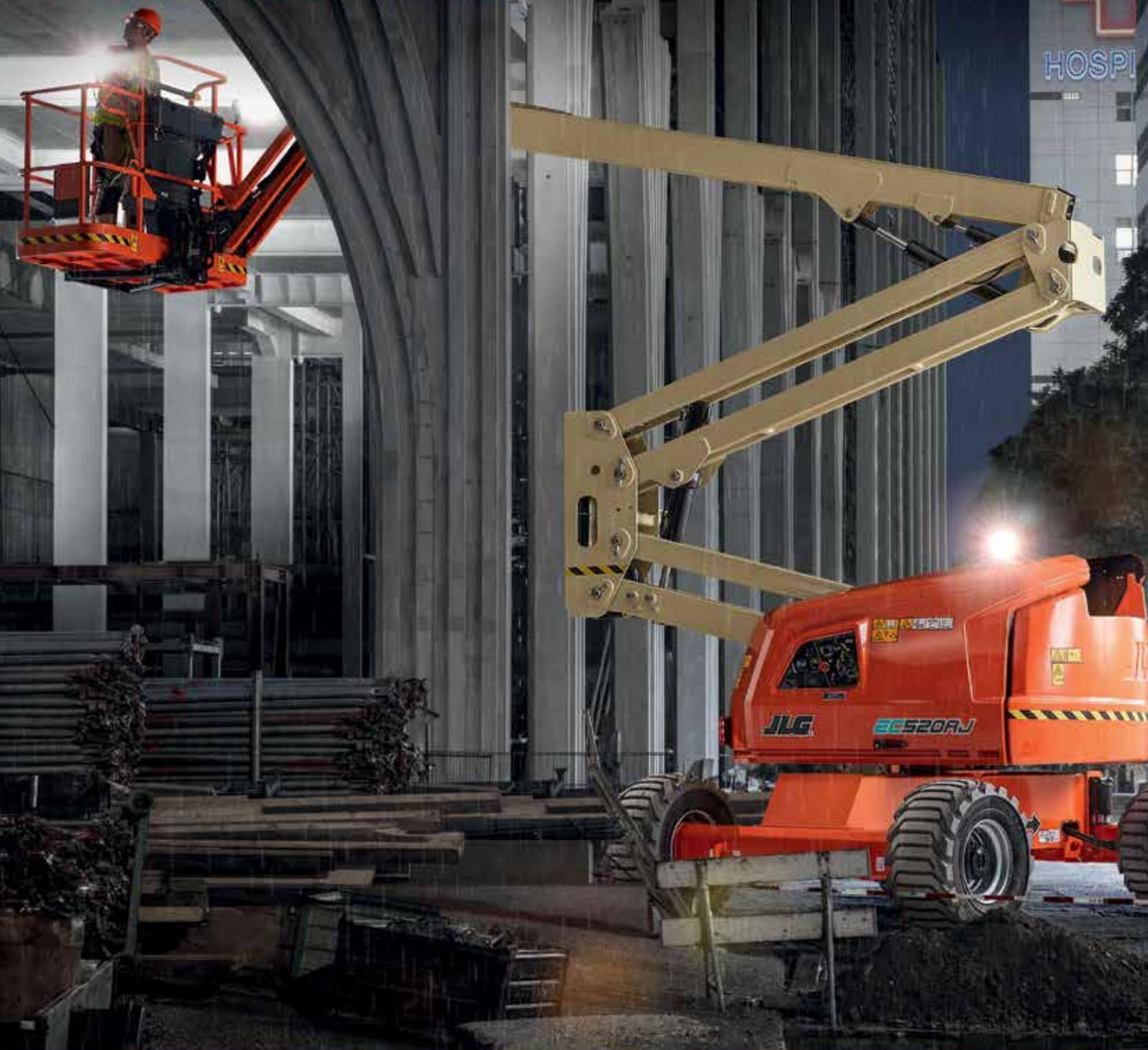
Now you can work in sensitive areas without disrupting the surrounding environment. Powered by safe, quick-charging lithium ion batteries and two electric motors, JLG® EC booms deliver clean operation and greater energy efficiency on any job site. Experience uncompromised performance with the flexibility to work inside or out with a single machine.
