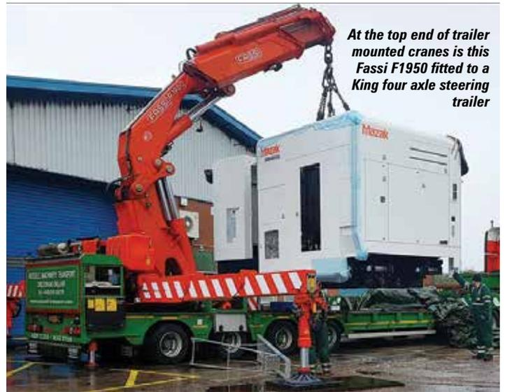
At the top end of trailer mounted cranes is this Fassi F1950 fitted to a King four axle steering trailer
