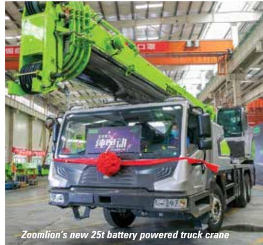
Zoomlion's new 25t battery powered truck crane
