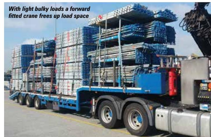
*With light bulky loads a forward fitted crane frees up load space*
