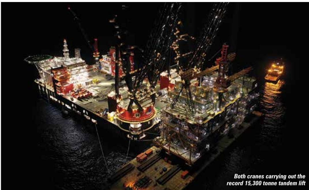
Both cranes carrying out the record 15,300 tonne tandem lift
