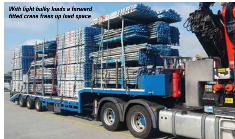
*With light bulky loads a forward fitted crane frees up load space*
