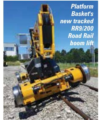
The superstructure also includes automatic levelling allowing it to level up on rail inclines or banked tracks of up to 180mm or eight degrees. It can also be used as a regular self-propelled boom lift, but with a slightly reduced 8.5 metre working height and an outreach of 4.3 metres and can work on side slopes of up to three degrees. With the riser fully elevated the RR9/200 has zero tailswing so that it can be used alongside a live second track.
