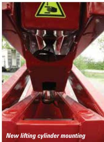
*New lifting cylinder mounting*
