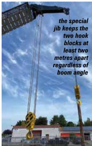
*the special jib keeps the two hook blocks at least two metres apart regardless of boom angle*
