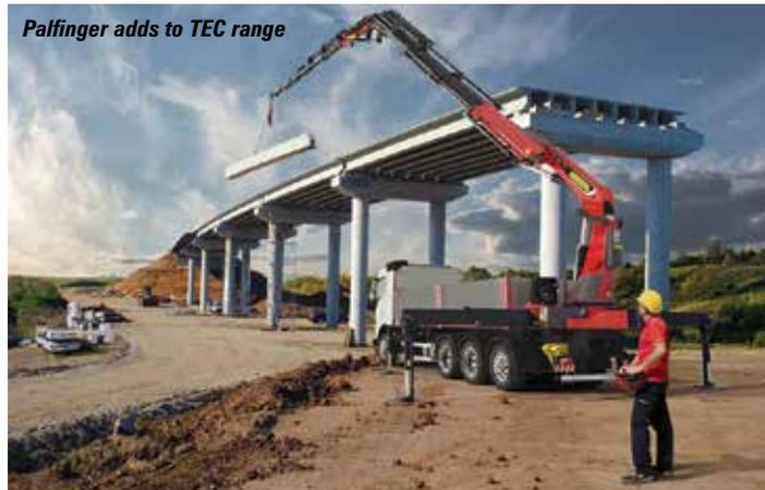
Tec 7s - DPS Dual Power System for full lifting power in jib mode - DPS-Plus for the TEC 5, and DPS-C for the TEC 7 - along with the HPSC-Plus module which monitors the crane bed tilt to provide increased capacities and improved stability by taking the load on the truck into consideration. This allows higher capacities when fully laden which reduces as it is unloaded.
