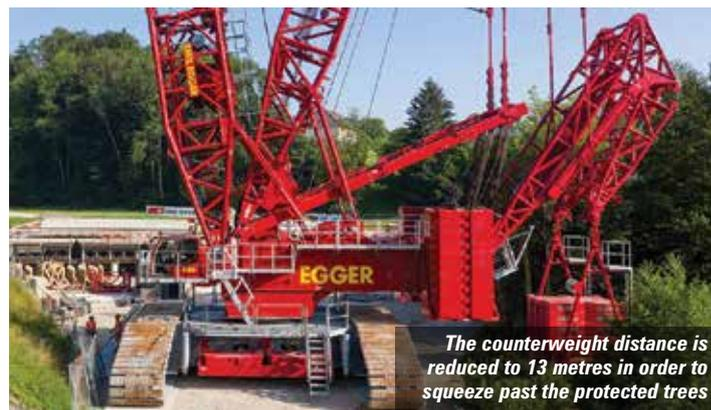
The counterweight distance is reduced to 13 metres in order to squeeze past the protected trees
